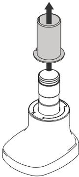
2.2 To remove rotation ring press down on front edge and lift.
