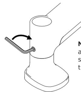
**Note:** Check the arm rotation is smooth after tightening.
