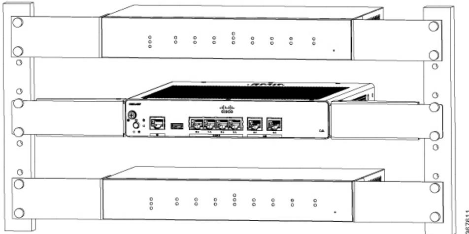
**Note** Allow at least one rack unit (1RU) of vertical space between routers. More clearance may be required when stacking multiple products in the rack that could build up heat in the rack. Ensure that the ambient around the router is within the ambient temperature specified in [Table 3: Ambient Temperature of SKUs, on page 11](#).
