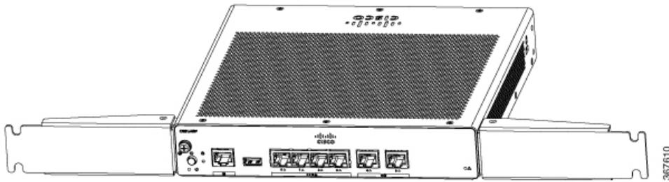
Figure 12: Router with Bracket Attached to Front Panel
