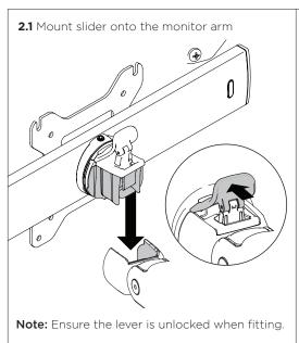
**2.2** Ensure that the slider is seated fully into the receptacle at the end of the monitor arm. There should be **no** gap.
