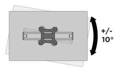
**3.3 (Optional)** Monitor rotation tension may be adjusted by tightening or loosening a small screw with the provided allen key.
