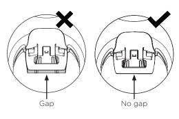
**2.3** Push the lever down to secure it to the arm assembly
