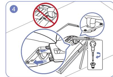
Fasten the screws at the bottom of the stand neck.
