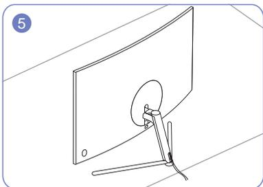
Tie up the connected power supply and the data cable then cover the COVER-REAR SUB as shown in the figure.
