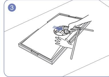
Lift and remove the stand in the direction of the arrow as shown in the figure.
