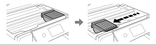
7. Push the tab to unlock the ink cartridge holder, and then remove the cartridge diagonally.
