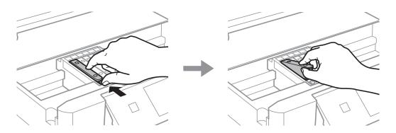
Insert the ink cartridge diagonally into the cartridge holder and gently push it down until it clicks into place. 8.
