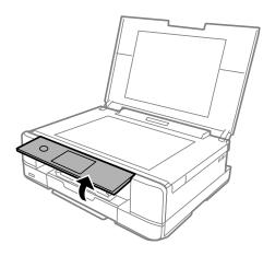
4. Loosen the screw with a flat-head screwdriver until the maintenance box cover comes off the printer.
