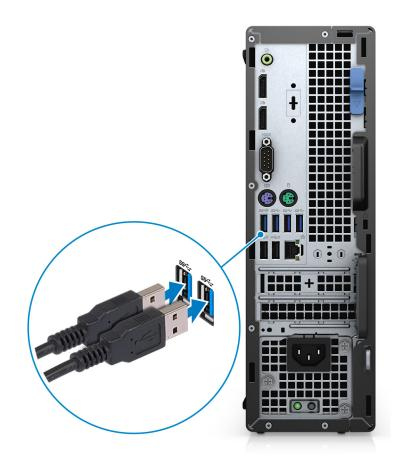
2. Connect to your network using a cable, or connect to a wireless network.
