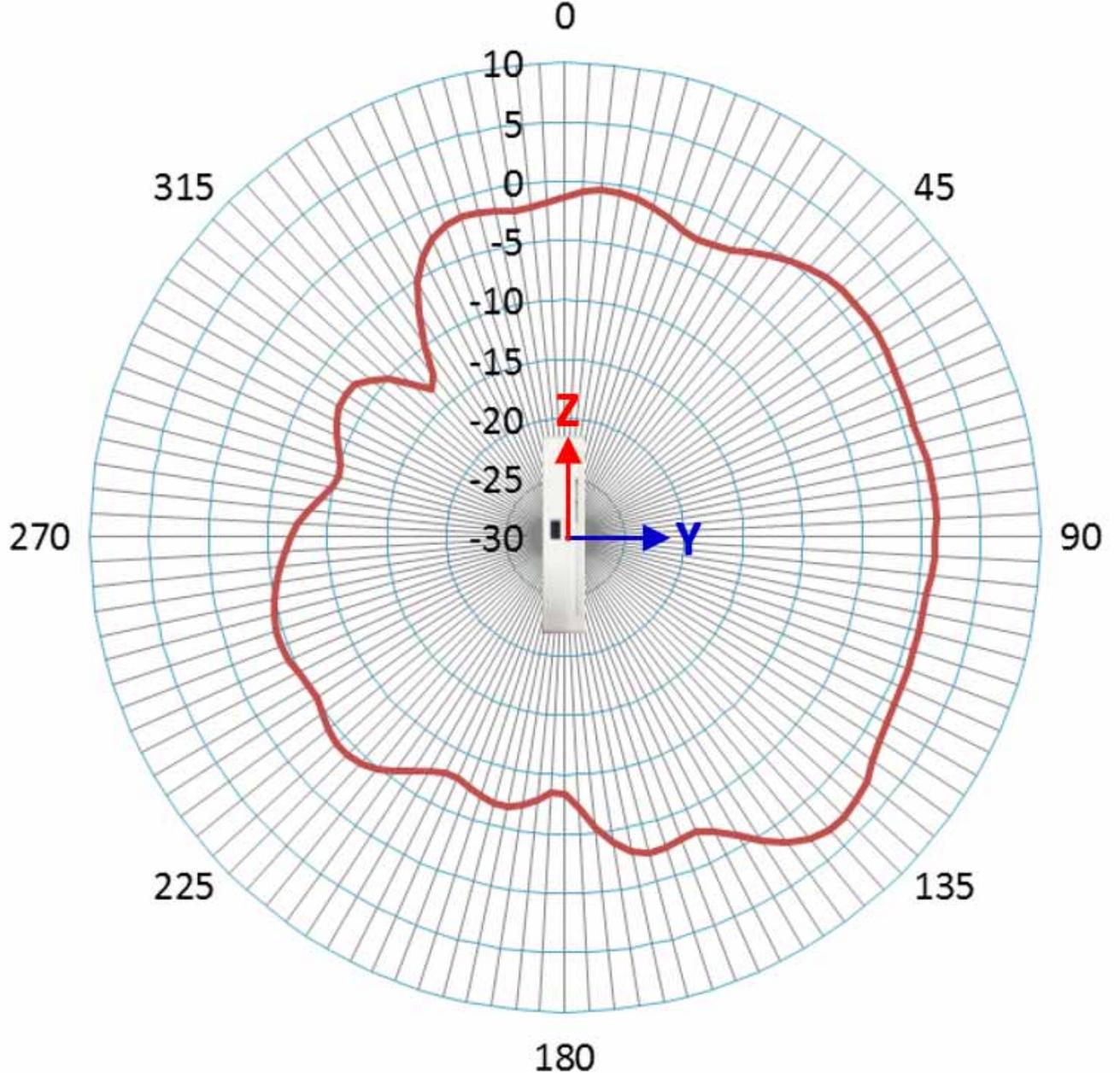
Figure 5 C9105AXW and C9105AXWT — BLE Antenna — Azimuth
