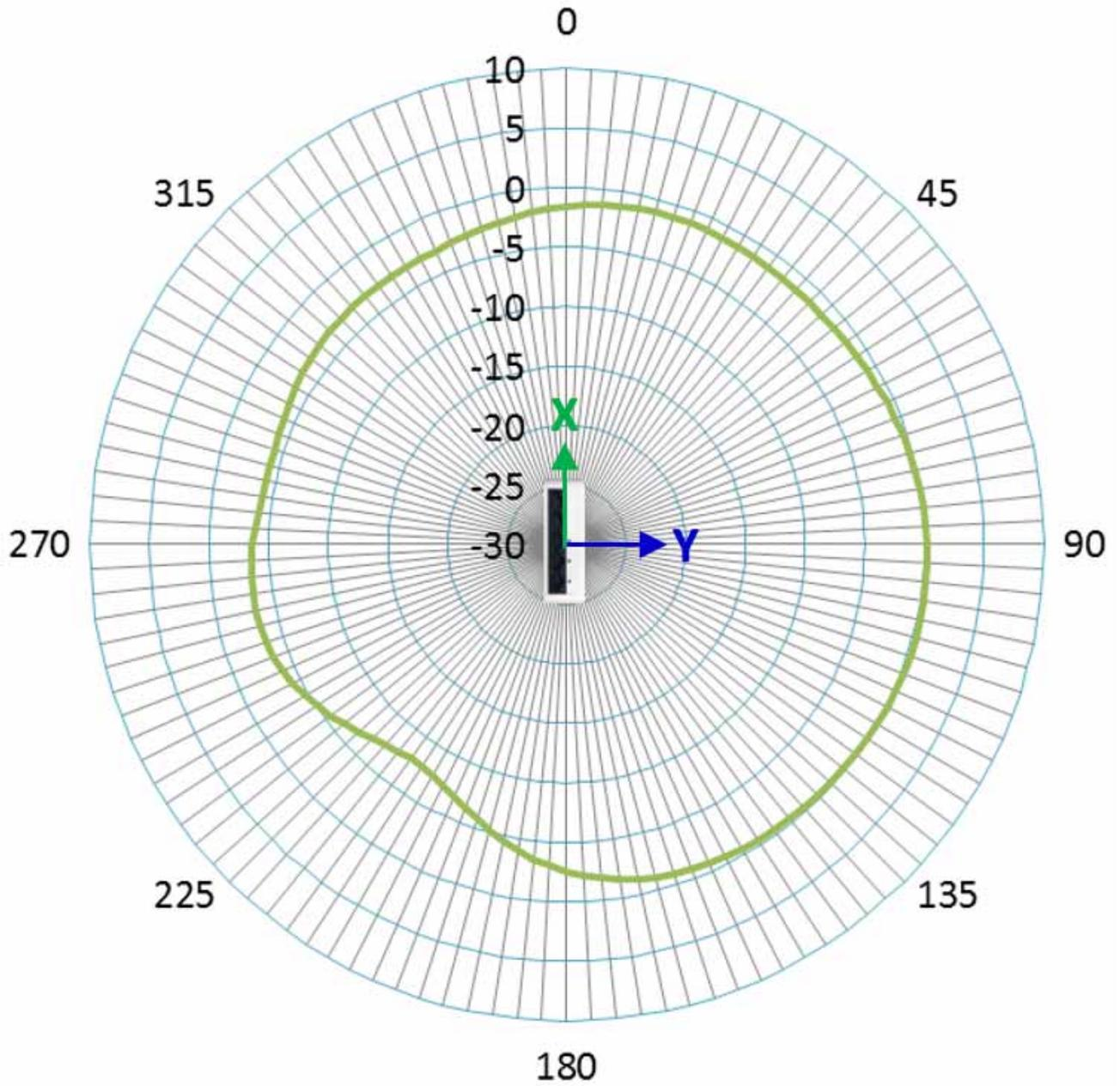
Figure 2 C9105AXW and C9105AXWT — Dual-band Antenna (2.4 GHz) — Elevation
