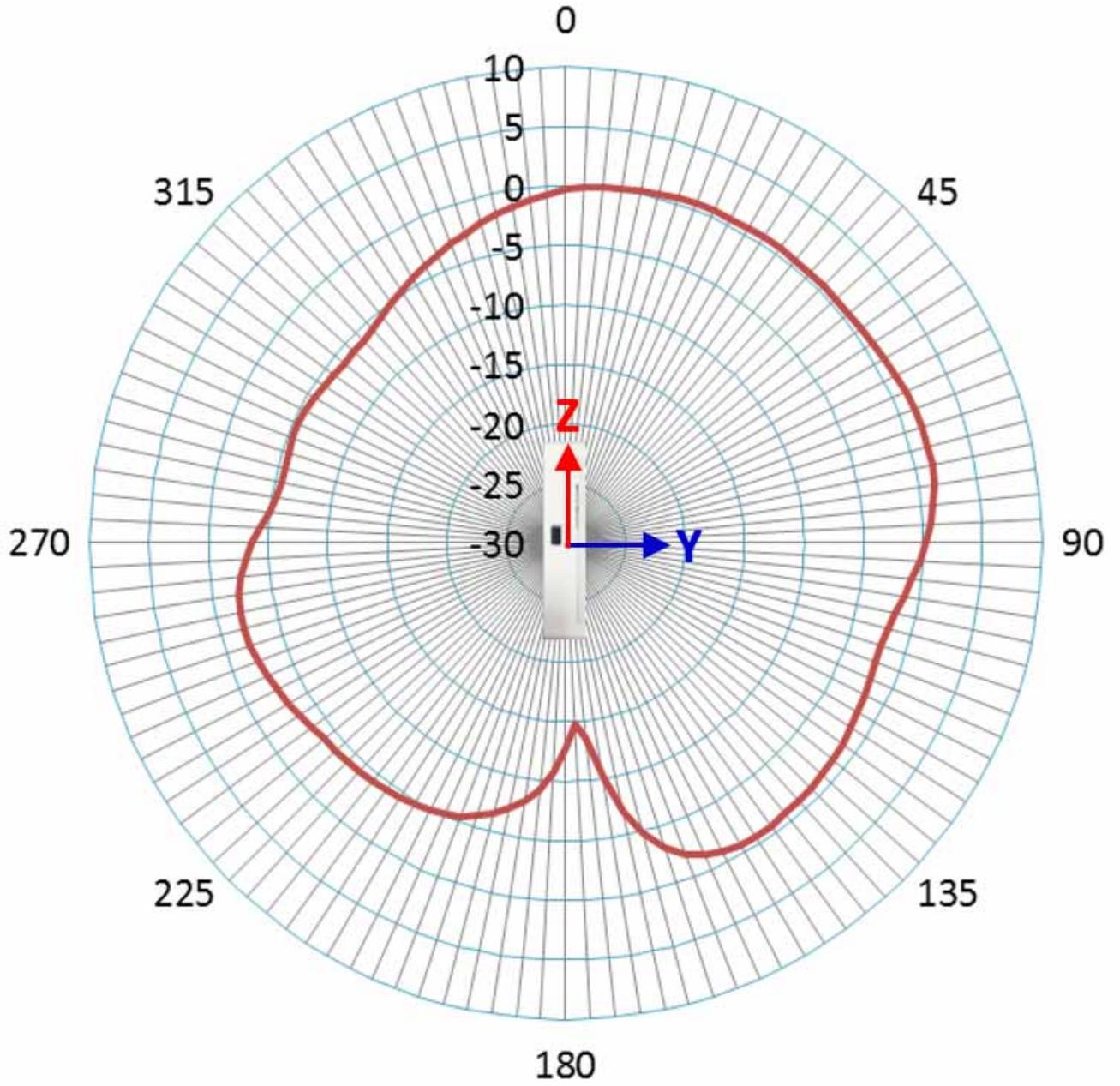
Figure 3 C9105AXW and C9105AXWT — Dual-band Antenna (5 GHz) — Azimuth
