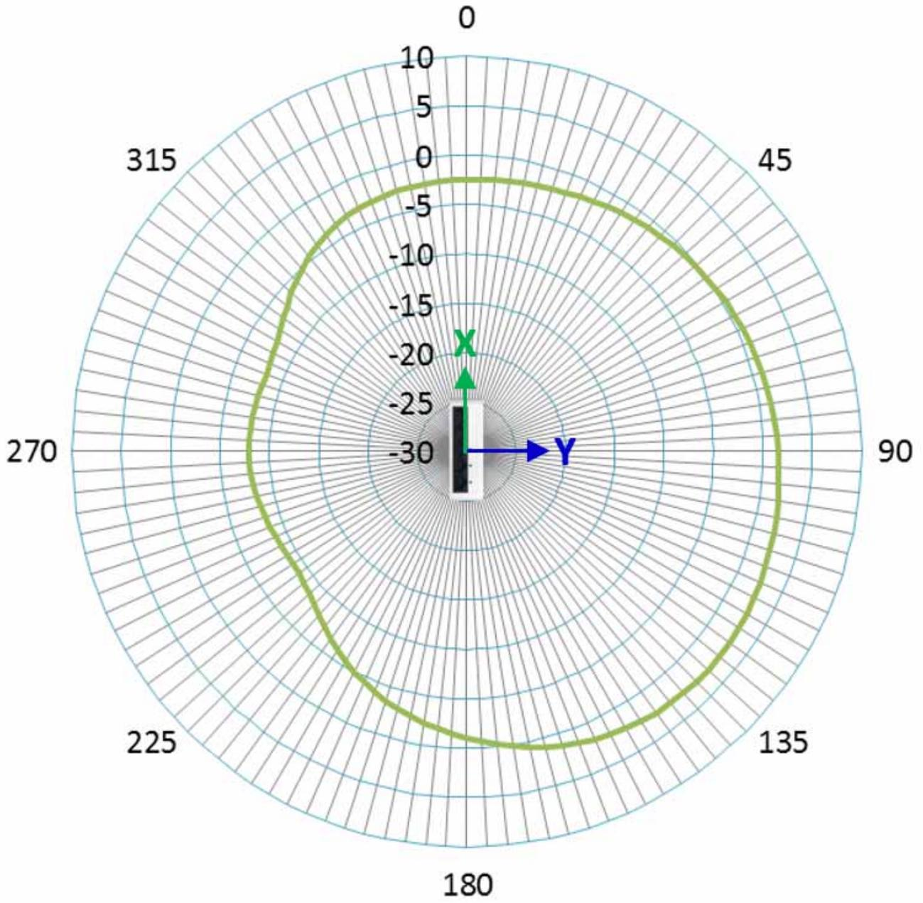
Figure 6 C9105AXW and C9105AXWT — BLE Antenna — Elevation
