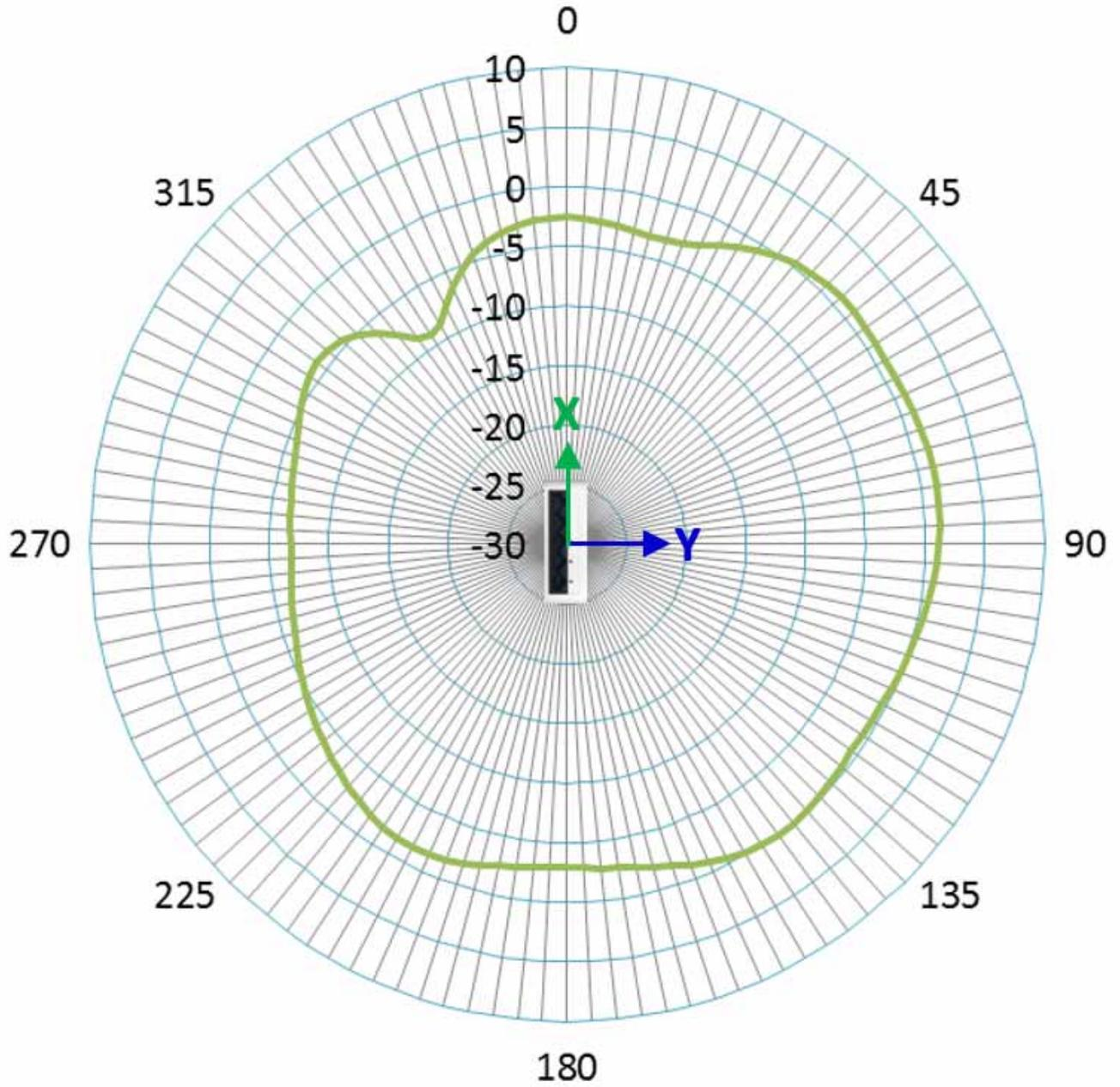
Figure 4 C9105AXW and C9105AXWT — Dual-band Antenna (5 GHz) — Elevation
