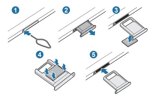
Insert the ejection pin into the hole on the tray to loosen the tray.
