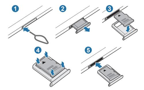
1 Insert the ejection pin into the hole on the tray to loosen the tray.
