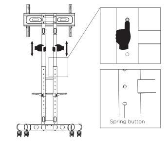
9.2 Person "A" holds the top section of the telescopic column. Person "B" depresses left and right spring buttons on column by using thumbs, so that person "A" can move top of column down or up to desired height.
